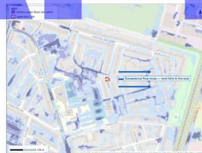
Figure 4 - Surface water exceedance flow route
